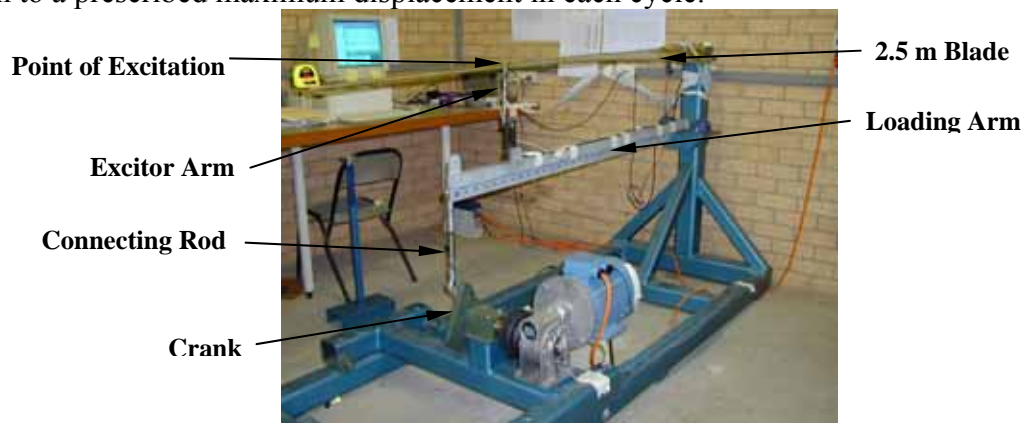
Figure 1 Fatigue test rig.
