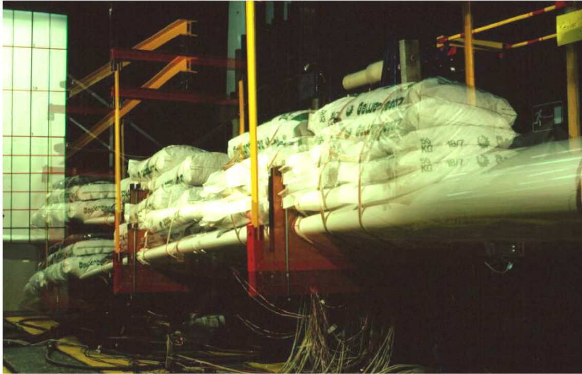
Fig. 5. DEBRA 25 blade in test bed for service life investigation.
