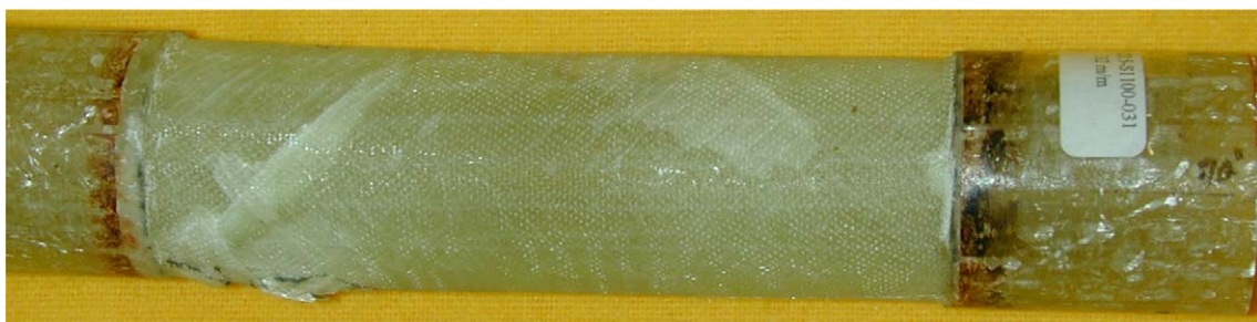
Fig. 13. Improvement of failure mode with tapered overlap.
