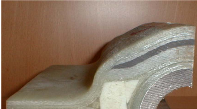
Fig. 19. Picture of hybrid laminate in a stud joint [25].
