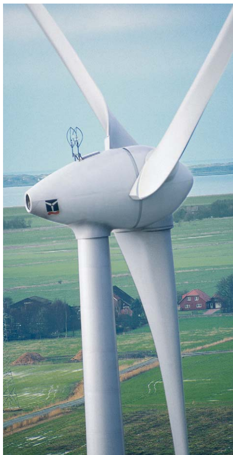
Composites are not only used to manufacture the turbine's rotor blades, they can also be used to produce the drive shafts. (Picture courtesy of Enercon.)
