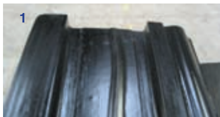
1. View of the contra mould flange zone showing the profile which must be laminated successfully.
