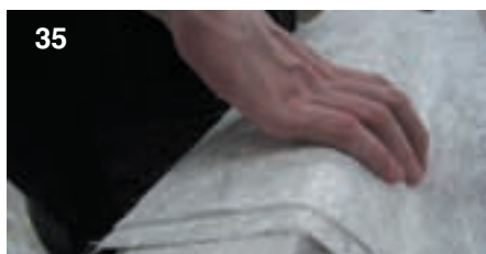
35 Apply the final 2 layers over the main mould cavity and continue up and over the Mastercored flange, right up to the mould edge.
