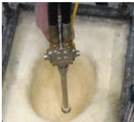
Injection into composite matched mould
