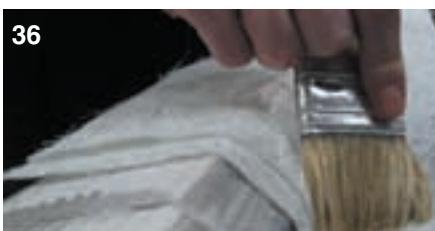
35 Apply the final 2 layers over the main mould cavity and continue up and over the Mastercored flange, right up to the mould edge.
