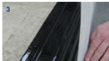
3. Tissue layer is carefully smoothed into flange detail, over the dry gel coat.
