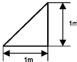
Use this template to measure fiber direction of rovings in the  $\pm 45^\circ$  and  $90^\circ$  directions according to the following drawing.
