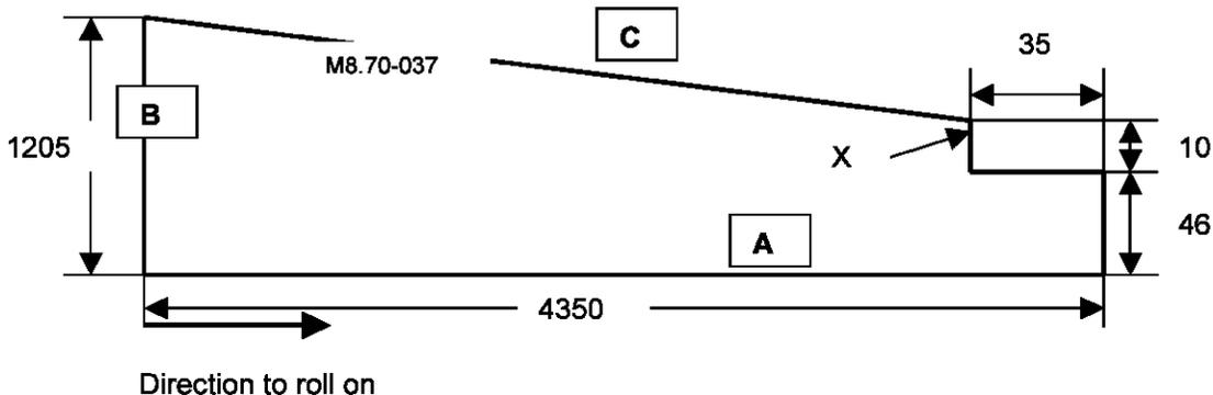
Roll off the fabric layer 24 hours later and compare the dimensions given in the drawing with the sizes from the layered fabric. The X-Point is the fix point to start measuring in the length and the width.
