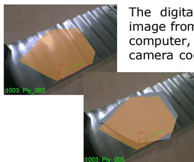
The digital camera coordinates and the live video image from the camera are both fed continuously to a computer, via suitable interfaces. By using the digital camera coordinates, the supplied Placement software
