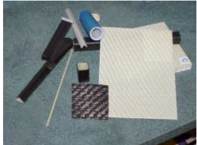
Figure 9: Various Forms of Continuous Fiber Reinforced Thermoplastics Including Direct and Post Formed Pultruded Profiles, Filament Wound Tube, Consolidated Plates and Sandwich Structures
